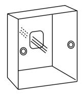
2. Fix back cover to the holder. After that, connect communication wire to CON1 port of wired controller. Finally put the front cover of wired controller to back cover to complete the installation.
