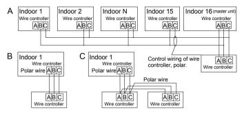
There are three methods to connect wired controller with the indoor units
