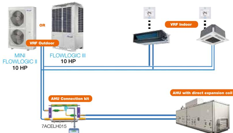
5 HP (14kW) < Connected AHU capacity ≤ 10 HP (28kW)
