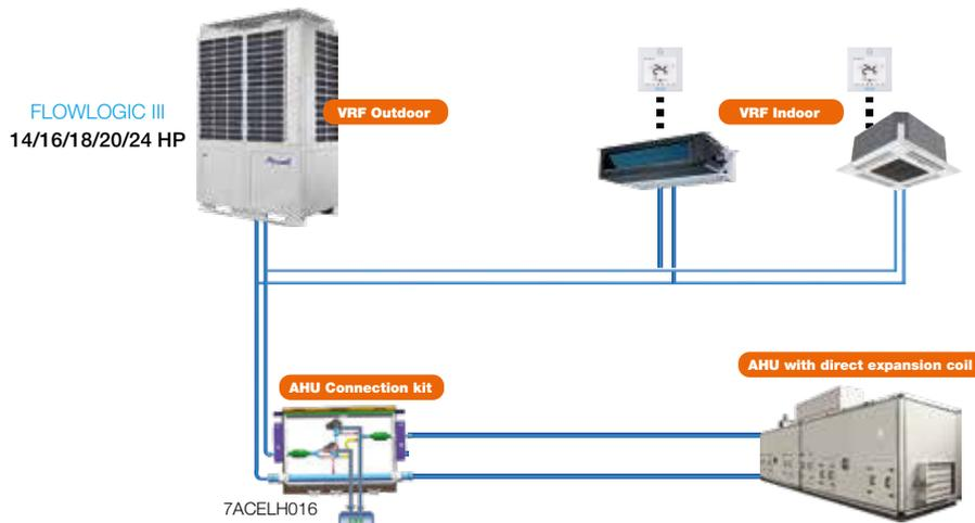
10 HP (28kW) < Connected AHU capacity ≤ 20 HP (56kW)
