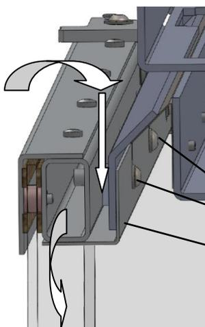
Above the glass panes, secondary air creates a film of air along them which reduces carbon deposits. A strip in the upper part of the glass has been installed to allow you to manage this air. To do so, unscrew the screws (\*) and lower (open) or raise (close) the strip.
