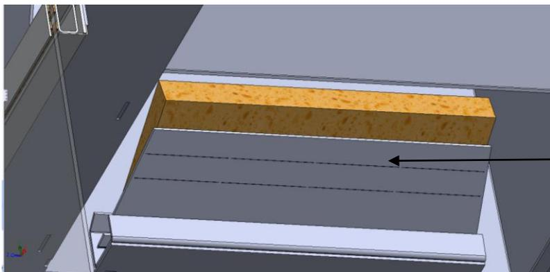
The reflectors are placed on a divisible steel sheet. It is therefore possible to increase the smoke flow surface area by breaking the micro-seams of the divisible sections; this adjustment must only be carried out by the fitter.
