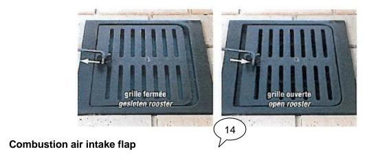
The combustion air intake flap is an optional extra which can be placed upstream of the adjustable air grate.
