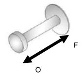
To increase the incoming air flow rate, pull the control lever.
